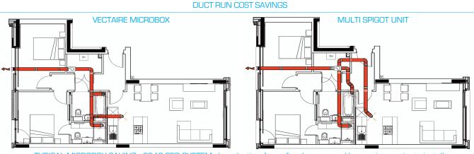
TYPICAL MICROBOX SAVING - £249 PER SYSTEM - less ducting, fewer fire dampers and less coring, easier to install
