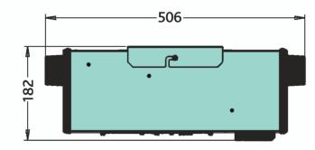
N.B a clearance of at least 200 mm should be allowed on each side of the cabinet for access to the interior
