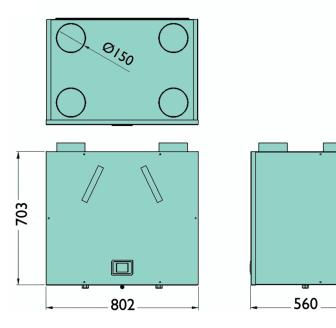
**N.B** a clearance of at least 200 mm should be allowed on each side of the cabinet for access to the interior
