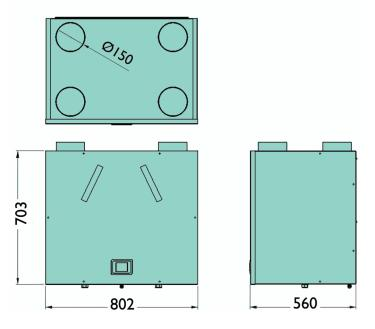
**N.B** a clearance of at least 200 mm should be allowed on each side of the cabinet for access to the interior
