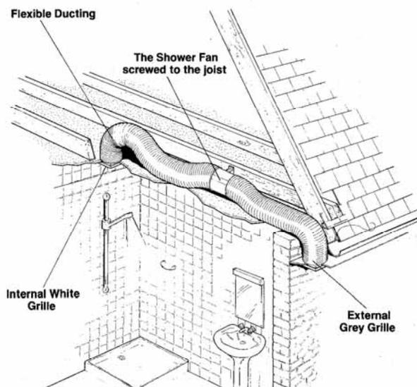
3. An adequate supply of fresh air must be provided if the fan is to be fitted in a room containing a fuel burning appliance which is not of the balanced flue type.
