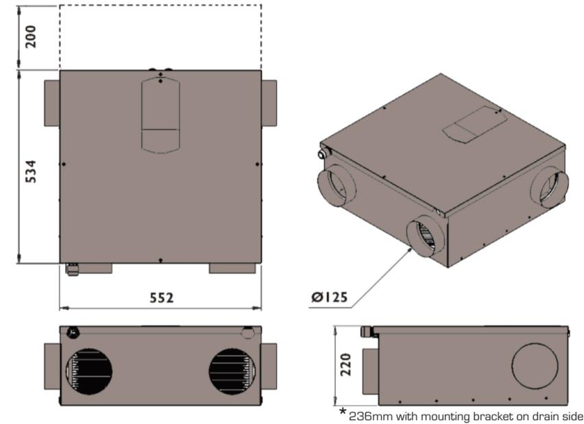
**N.B** a clearance of at least 200 mm should be allowed at the rear of the unit in order to replace filters. A clearance of 220mm should be allowed at bottom of unit when installed for access to the heat exchanger
